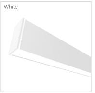
Continuous suspended/surface mounted IP 65 linear aluminium profile 44 x 77mm (WxH) with optional stand-alone surge protection. Replaceable quick fit gear tray modules with safety lanyards. Samsung LED package, 3 MacAdam steps. Integral driver with current selection. Delivered efficacy rating up to 120lms/W (CRI80), L90 B10 75,000h. PolyLED diffusers with no visible spotting and uniform appearance. Minimum 7 year warranty.
